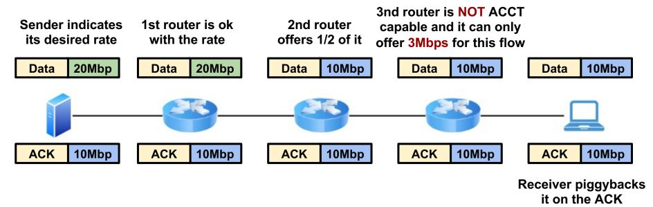
ACCT detects that the 3rd router is the bottleneck it then regulates its sending rate on that basis
