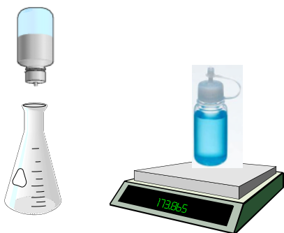
Graphic 1: Gravimetric Titration with a Polymer Controlled Drop-Dispensing Squeeze-Bottle and a 2-Place Digital Balance
